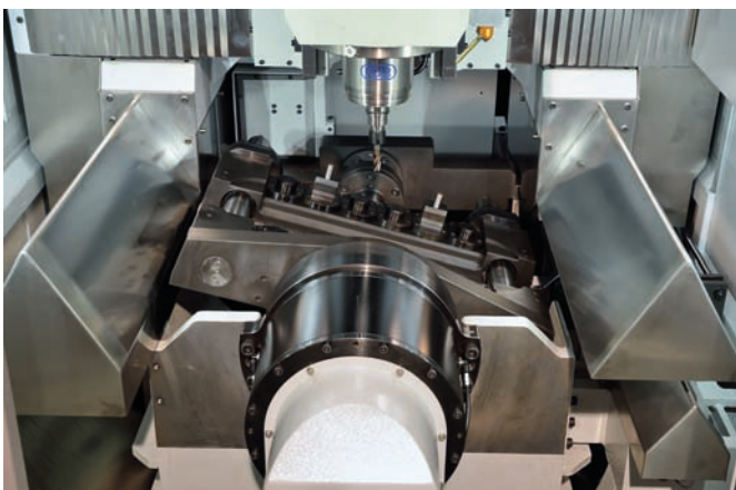
Rotary Vice Positioned Tilted with Respect to the Rear Face
