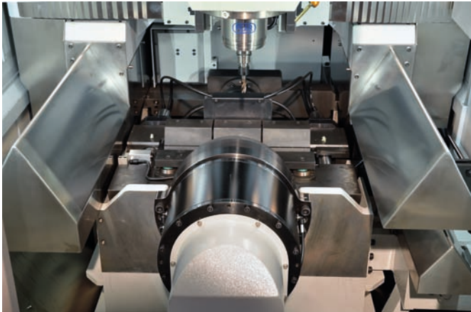
Rotary Vice Positioned Tilted with Respect to the Front Face
