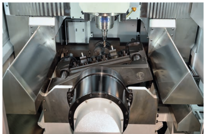
Rotary Vice Positioned Tilted with Respect to the Rear Face
